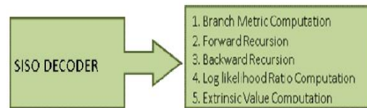
Figure 4 main task of SISO decoder
